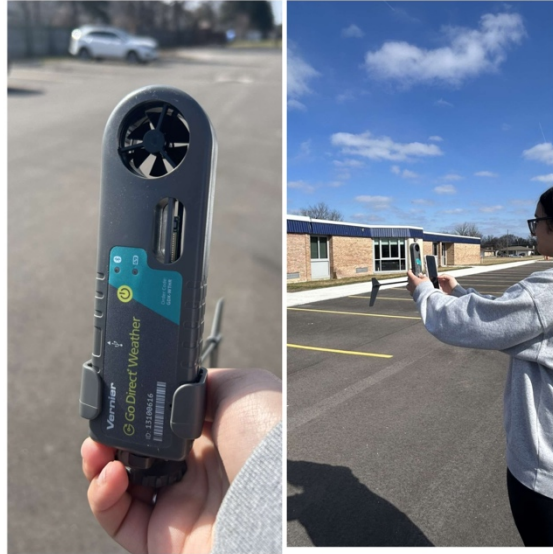
Figures 5 and 6. Vernier Go Direct Weather device. The image on the left shows the Vernier Go Direct Weather Device that was used to measure the wind speed. The image on the right shows a researcher taking data using the device.
