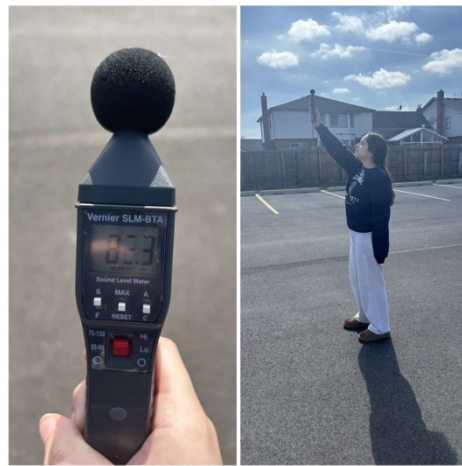
Figure 3 and 4. Vernier Sound level meter. Image to the left is an up-close picture of the Vernier Sound Level Meter that was used to measure noise levels. The image to the right shows a researcher using the Sound Level Meter.
