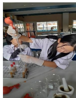
figure B.2.8 Aspirate the clay solution into the test tube.
