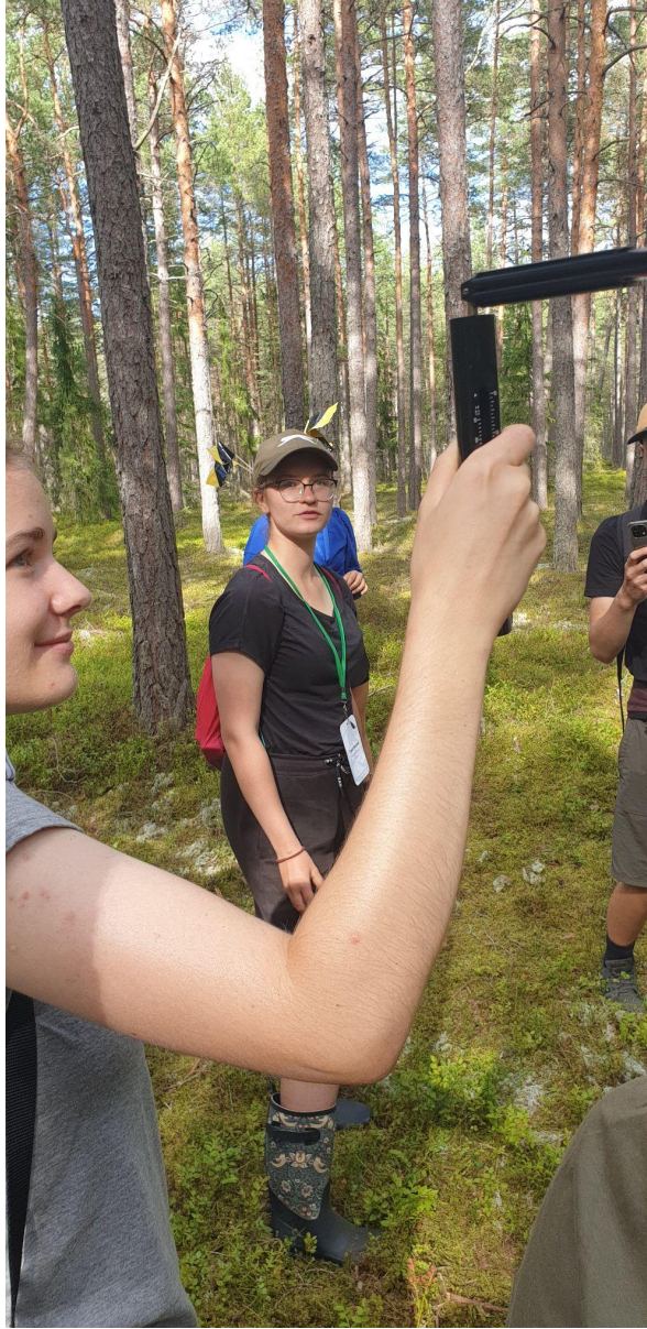
Figure 4. Measuring humidity with a psychrometer.
