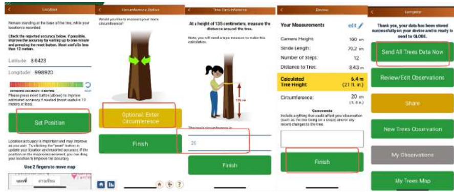
Figure 3. The GLOBE Observer: Trees App. (a) Choose Protocol: Trees >> New Trees Observation >> Choose the date, time, latitude & longitude and select the following surface conditions. (b) Take a photo: choose your tree and your positions while counting your steps (c) Set position >> Measure your tree circumference >> Finish and send your tree measurement to the GLOBE App.
