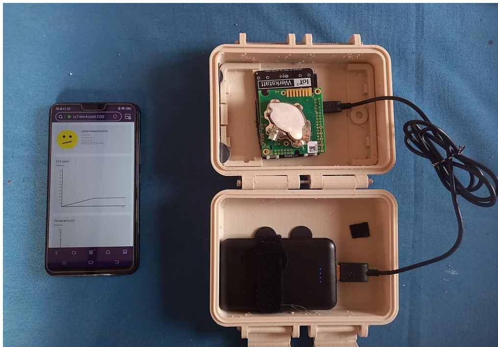
Figure 8 CO 2 sensor connected to mobile phone via Wi-Fi. Phone displaying CO 2 data.
