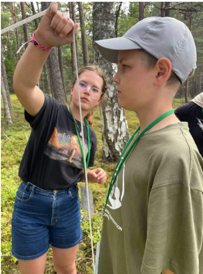
Figure 10. Measuring eye height for clinometer measurements.
