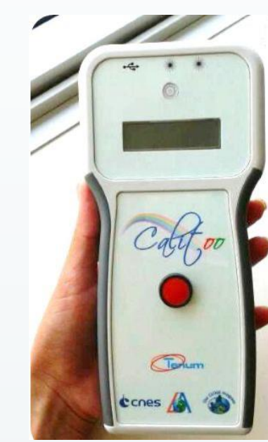
Measure the Aerosol Optical Thickness levels using the Calitoo Sun Photometer
