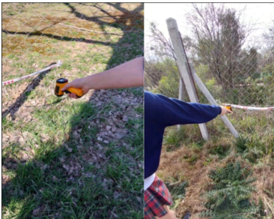
Image N°16 | Students measuring surface temperature using a handheld infrared thermometer
