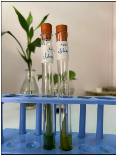
Image (8) comparison of the results of detecting Co2 emission from the plant in the control and experimental sample after three months using the Bromothymol detector.
