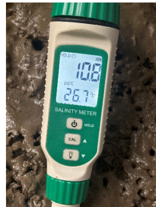
Measuring salinity using a Salinity meter
