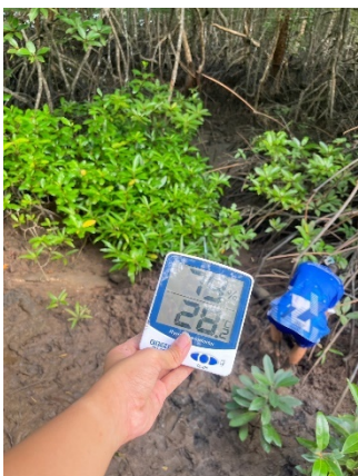
Measuring air temperature and humidity using a DIGICON TH-02A.
