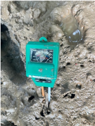
Measuring pH using a Soil pH Meter SPM05.
