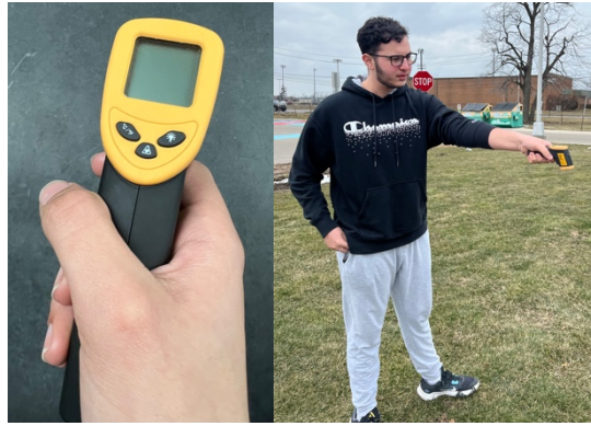
Figures 3-4. Infrared Thermometer. Figure 3 (left) is a closeup photo of the Etekcity Lasergrip 774 infrared thermometer. Figure 4 (right) is an image of a student researcher using the infrared thermometer to collect ground temperature measurements.
