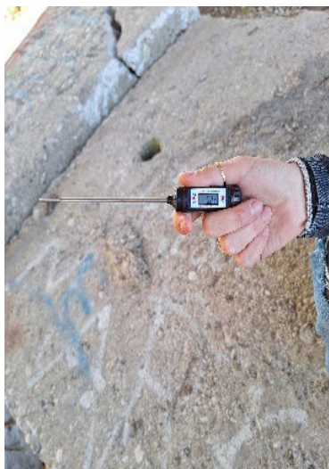
Figure 22. The Air Temperature Measurement
