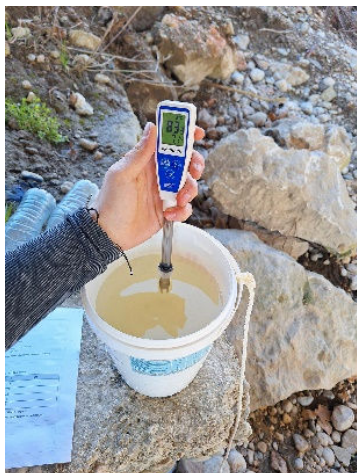
Figure 26. The Water pH Measurement
