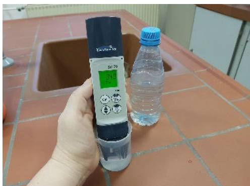
Figure 25. The Electrical Conductivity Measurement
