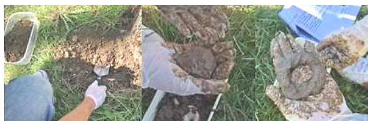
Figure 19. Taking a soil sample and determining the type of soil in the field.
