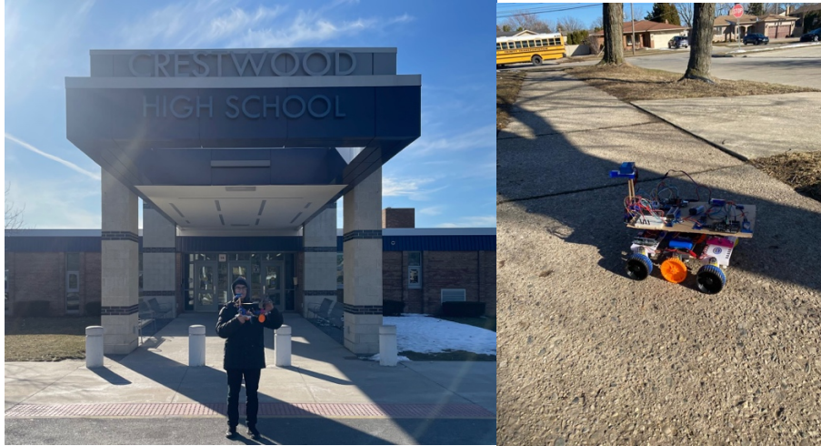
Figure 10 and Figure 11. TerraRover 2's Use at Crestwood High School. Images above greatly shows TerraRover 2 at Crestwood. Throughout the research, the TerraRover 2 was being driven to efficiently collect data for particulate matter, carbon monoxide, carbon dioxide, ultraviolet light, sound and GPS all around the researchers' sites.
