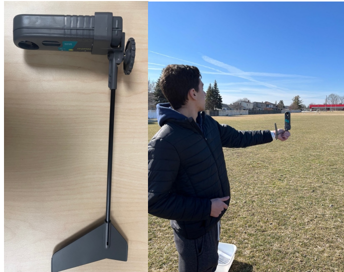
Figure 4 and Figure 5. Vernier Go Direct Weather Device. Image on the left shows the Vernier Go Direct Weather Device that we used to take most of our data. Image on the right shows a Dearborn Heights researcher taking data using the device.
