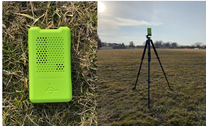
Figure 5-6: Weather instrumentation. The data was recorded on a PocketLab Air (left) attached to a 1.2 meter high tripod (right). Figure 6 (right) shows the PocketLab Air 1.2 meters high collecting surface ground weather and particulate matter data continuously every 15 seconds. Researchers were careful to level the instrument to be certain that wind speed and direction were accurately recorded. Weather data was not collected directly at the surface to avoid wind turbulence which could have affected the results.
