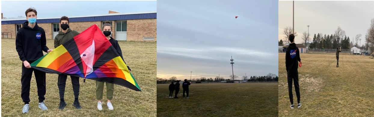
Figure 7-9: Kite Data Collection. After the PocketLab Air was finished collecting ground data, the researchers sent the PocketLab up 122 meters into the air to take data once more. Figure 7 (left) shows the researchers checking weather conditions to deem if flying is suitable. Once a decision is reached, the researchers flew the kite (middle) with the PocketLab attached. When the PocketLab Air is finished collecting data, the researchers take down the kite (right) and transfer all the data into Microsoft Excel.
