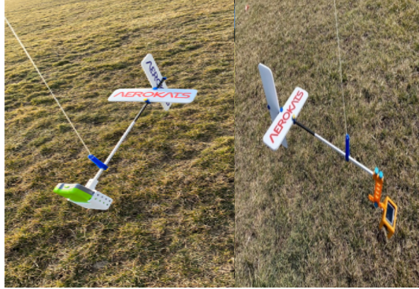
Figure 10-11: Aeropod Technology Used. The PocketLab Air was attached to a custom, 3-D printed Aeropod to collect PM and weather data 122 meters in the air (left). The Monocam was attached to the Monocam Aeropod and sent 305 meters in the air to capture an image of the field used for data collection (right).
