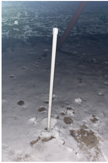
Figures 3, 4, & 5. Frost tube. Finished frost tube above ground (left), Installed Frost Tube (center), and Installing of the frost tube (right).
