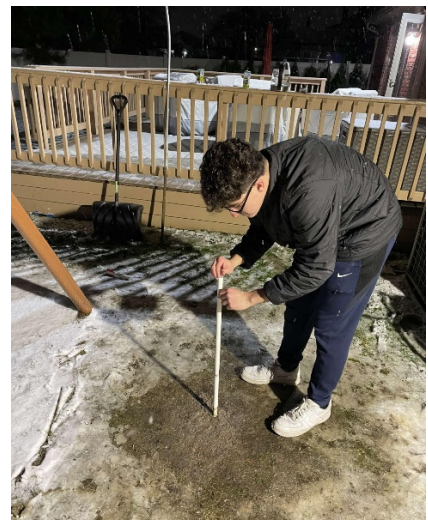
Figures 3, 4, & 5. Frost tube. Finished frost tube above ground (left), Installed Frost Tube (center), and Installing of the frost tube (right).
