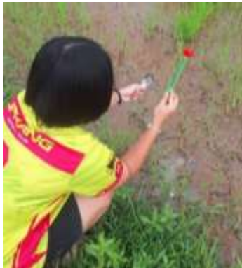
2. Measure the soil temperature in the rice field before cultivation, during cultivation (1st and 2nd cycles), and after cultivation.
