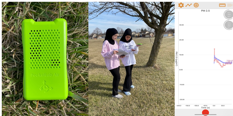
Figure 8-10. PocketLab Air was collected by one of the researchers waiting 3-5 minutes at shoulder length, while the other used a mobile device to collect the data of PM 2.5 and Ozone (middle). The green sensor (left) is what was used to gather this data on the PocketLab app. After this time period you can see that the data starts to become constant (right), at this point the researchers added this to the spreadsheet.
