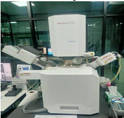
Thermo scientific Quattro S SEM (Scanning Electron Microscope / SEM)
