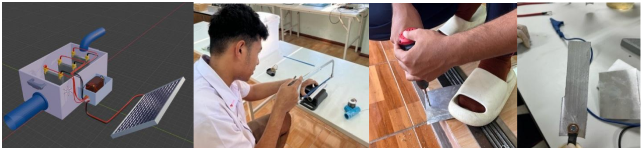
Model design Drilling electrode holes Cutting electrodes Electrode (Al)
