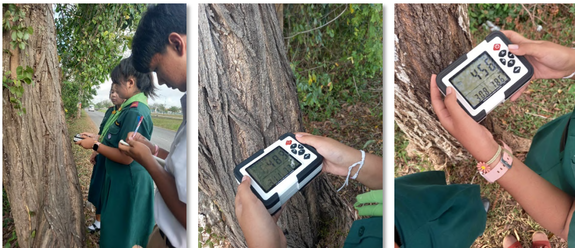
Figure 5: Measuring the temperature, relative humidity, and carbon dioxide level with the HT-2000 CO2 Meter
