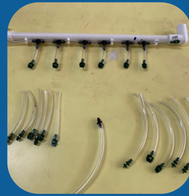
Figure 2: Installation of clear hose fitting for filling oxygen gas.
