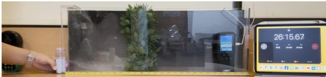
Fig. 17 The experimental setup. The white object on the left is a sprayer that can emit tiny water droplets as a source of pollutants. In the middle is a small wind tunnel. Fake tree strips are set up in the wind to bring up surface wetland vegetation. A pollutant sensor is set up on the right side of the wind tunnel, mainly to observe changes in PM2.5 concentration. On the right is a timer, which records the time of the experimental process.
