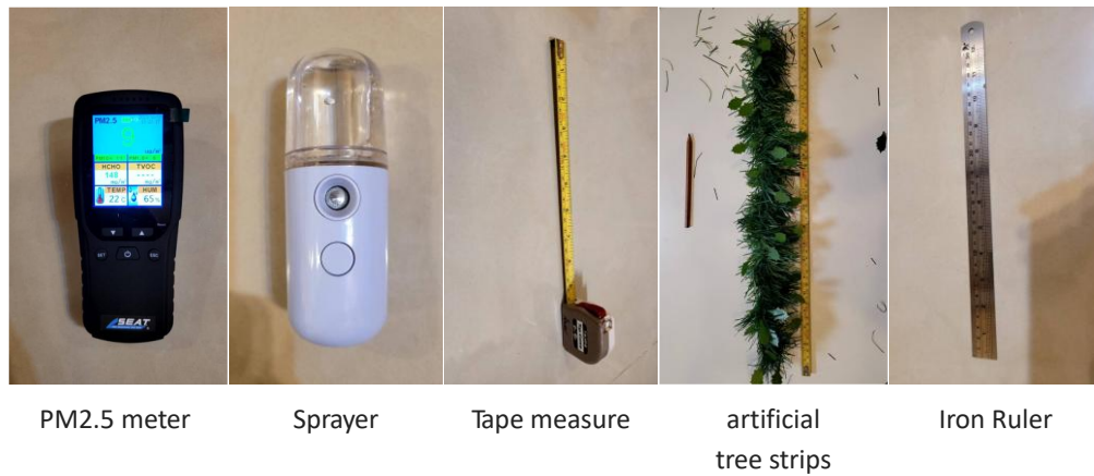
Fig. 15 Experimental equipment. From the left, PM2.5 meter: Records the concentration of pollution sources; Sprayers: as a source of pollution; Tape measure: Confirm the position of the artificial tree strips; Artificial tree strips: Simulating wetland vegetation; Ruler: Move the artificial tree strips.
