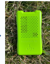
The PocketLab Air device used to take PM 2.5 and ground-level ozone measurements.
