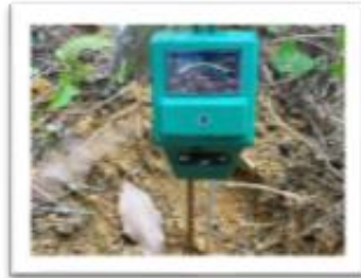
Figure 2: Soil Moisture Measurement
