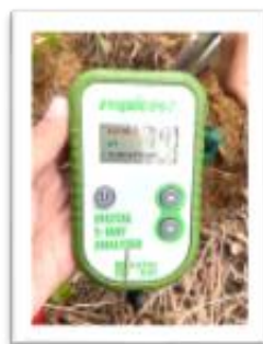
Figure 1: Soil Temperature Measurement
