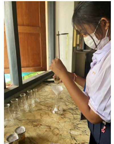
Figure 6: Filtering the sample for pH analysis.
