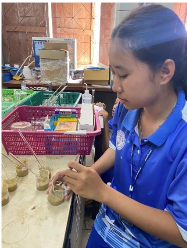
Figure 4: Mixing the sample for N, P, and K analysis.
