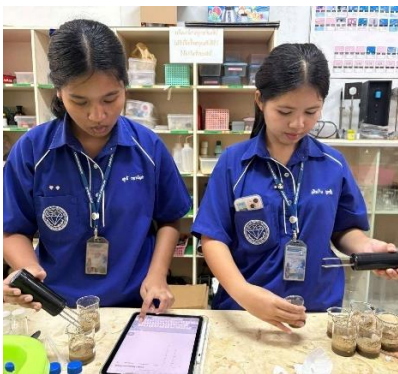
Figure 7: Measuring P and K values using a P K meter
