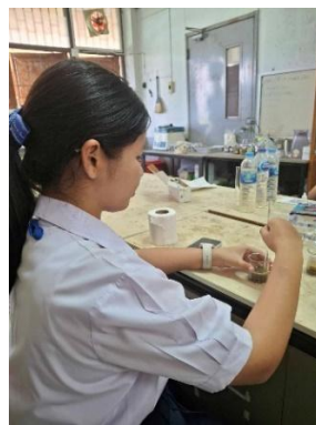
Figure 5: Stirring the sample for 30 seconds a specific number of times
