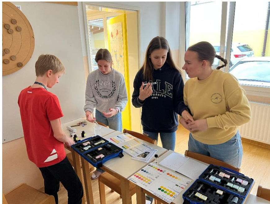
Figure 6: Determination of nitrate and nitrite using a water analysis case.
