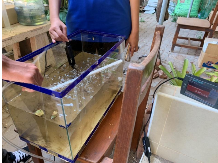
Figure 3: Testing different bubble diffuser heads for filling oxygen gas.
