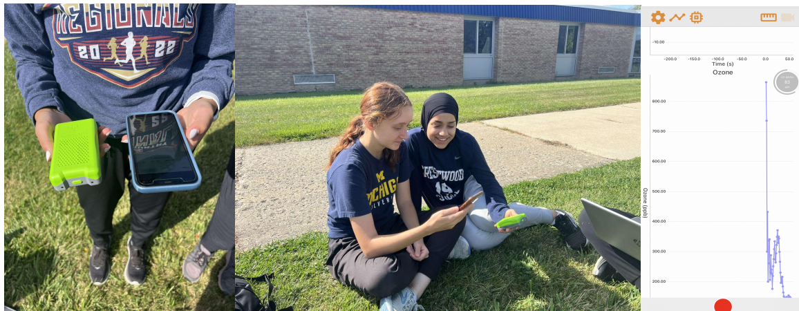
Figure 4-6. Pocketlab Air is a device that the researchers used at shoulder length for about 3-5 minutes for 96 consecutive days (first). A researcher held up and then read the ozone and PM 2.5 off the associated mobile app. After the researcher waited 3-5 minutes, the ozone data (right) stabilized and leveled off.
