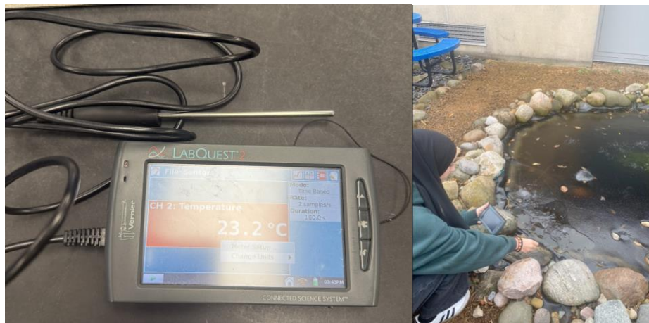
Figure 3 and 4. Water Thermometer. Figure 3 (left) is a close-up picture of the Vernier Temperature Probe. Figure 4 (right) is a student researcher demonstrating how they are collecting water temperature measurements with the water thermometer.
