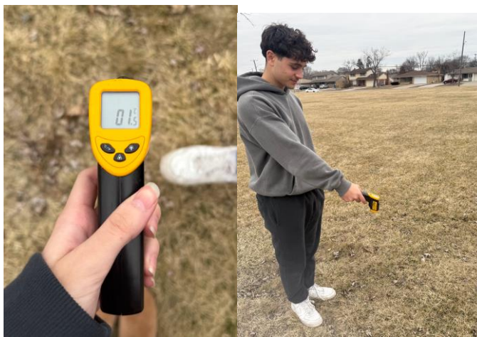
Figure 1 and 2. Infrared Thermometer. Figure 1 (left) is a close-up image of the Elekcitry Infrared Thermometer Laser Temperature Gun 774. Figure 2 (right) shows a student researcher using the infrared thermometer to record surface temperature measurements.
