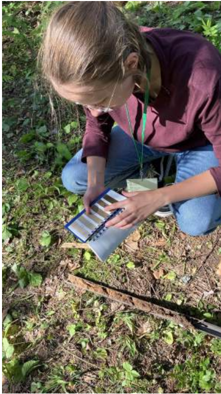
Figure 4. In the picture Kaili is using the soil colour chart to see the contents of the soil.
