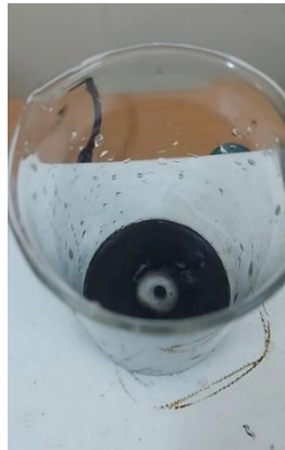
Image (3) Magnetic mixing capsule used in mixing sludge with cement
