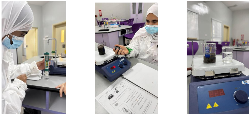
Image (2) The researchers apply acidity and conductivity protocols to the samples.
