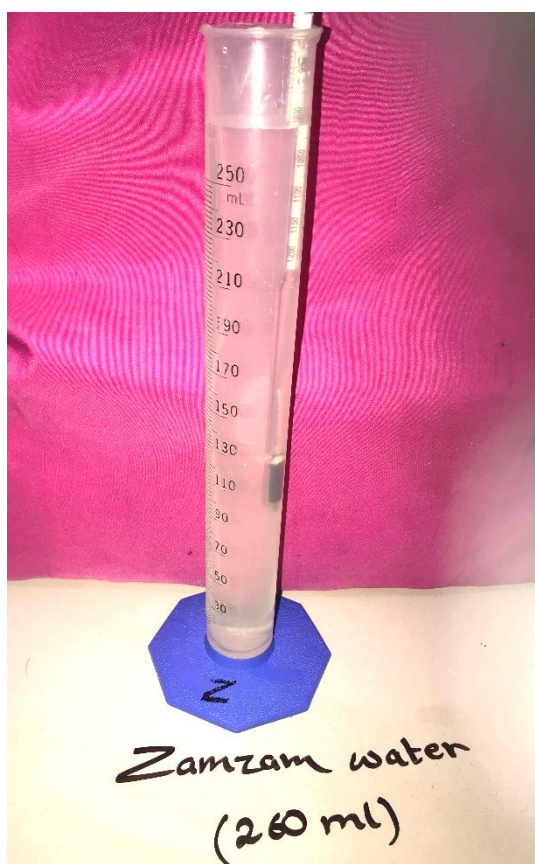
Figure (8): Measuring water specific gravity (Density) using a hydrometer (260ml bottled & Zamzam water).
