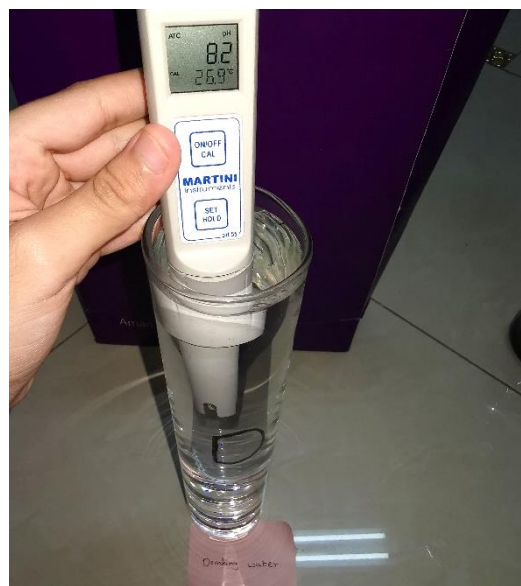
Figure (7): Measuring PH & temperature digitally by using acid device.
