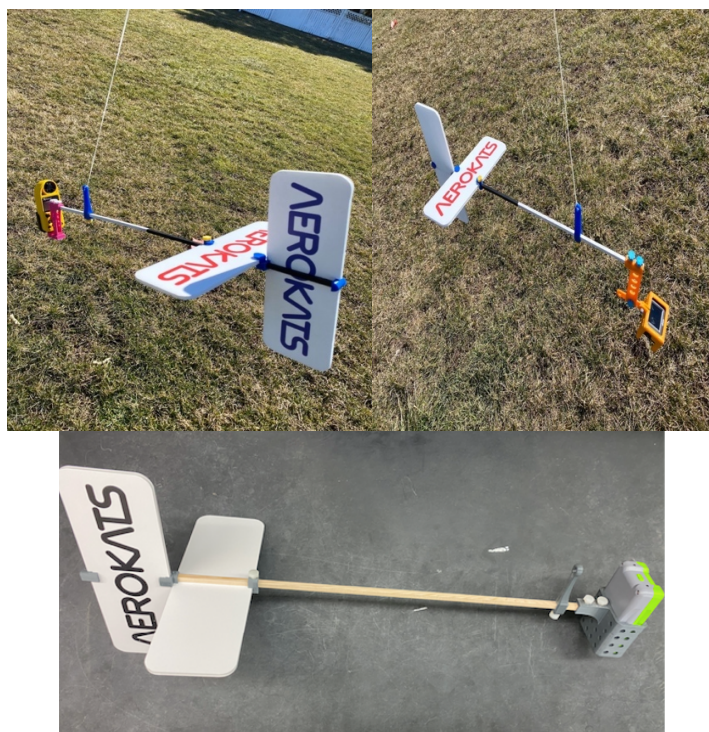
Figures 14-16: Aeropod Technology Used. Figure 14 (left) is the Profiler Kestrel Aeropod that was attached to the Levitation 7ft Delta Kite, where the Kestrel 5500 Weather Meter attached onto it continuously took data every 20 seconds at an altitude of approximately 122 meters in the air. Figure 15 (right) is the Monocam Aeropod with a Gitup Action Camera attached. This is how the researchers obtained their aerial shot- the Aeropod was sent about 274 meters in the air, where the Gitup camera took stunning videos and pictures of the site. Figure 16 (bottom) is the made to fit Aeropod that hold a Particulate matter reader, the Pocketlab Air. This Aeropod was made after special requests by the researchers, and is the first of its kind. The researchers hope to use this instrument to collaborate with student researchers in Thailand, and how we can compare particulate matter counts in each group's country.
