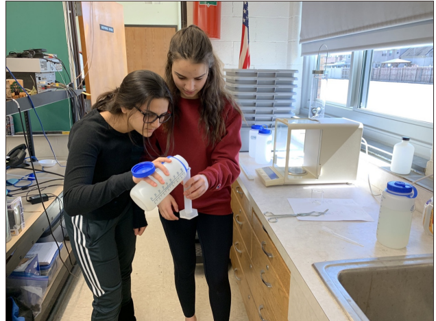
Figure 7-8: Figures 7 and 8 show two student researchers following protocol to obtain the water and measure total solids in the student lab.
