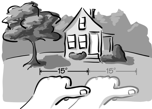
Figure GPS-RE-5: Using your hand to measure 15^\circ repeated trials. Hold your hand as steadily as possible. Focus on what is at the tip of your thumb, and then move your hand so that the back of your hand is now where your thumb tip was. Because you always take your hand with you, remember how you extended your arm and hand so that you can make future angle measurements. Practice positioning your hand and thumb so that you get a consistent number of "hands" between north and east or north and west. Now record what you see at the end of each hand width. After you feel
