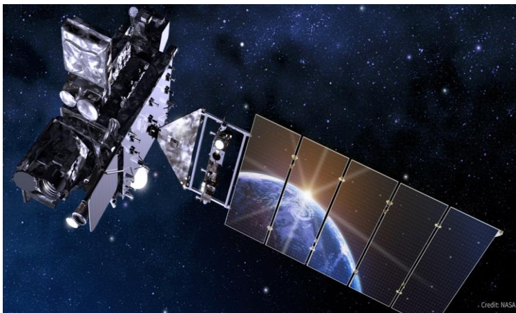
Figure 1. This is an artist’s image of GOES-16. One of the primary instruments on GOES-16 is the Advanced Baseline Imager (ABI). It collects data using 16 different spectral bands. The GOES-16 CSEP group used the ABI Band 13 during research.
