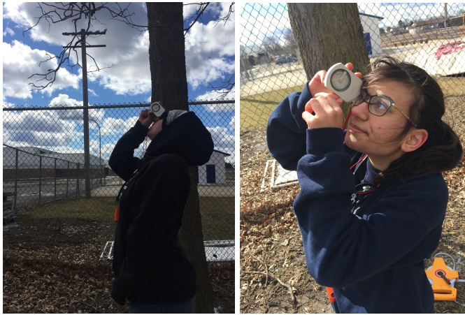
Figure 6-7: Figures 6 and 7 show the students using the clinometers following the GLOBE biometry protocol to measure the tree heights.
