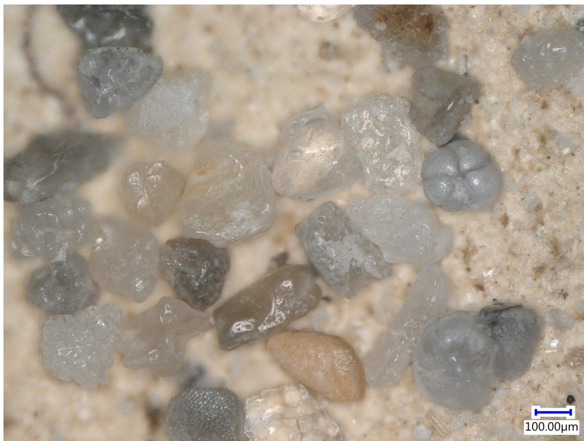
Figure 18. Courtesy Deakin University. High magnification images of naturally occurring sand shapes. Some of these shapes are clearly bio-derived (regular patterns on the surface and geometry) while some are just rock debris.
