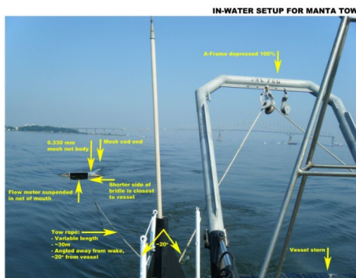
Figure 6. In-water setup for a manta tow. The vessel shown has an A-frame at the stern that is fully depressed, which supports a tow rope that is cleated to achieve an angle of ~20° between the vessel and the net to minimize interaction with the vessel's wake. The shorter side of the bridle should be closer to the vessel to help facilitate avoidance of sampling the wake.
