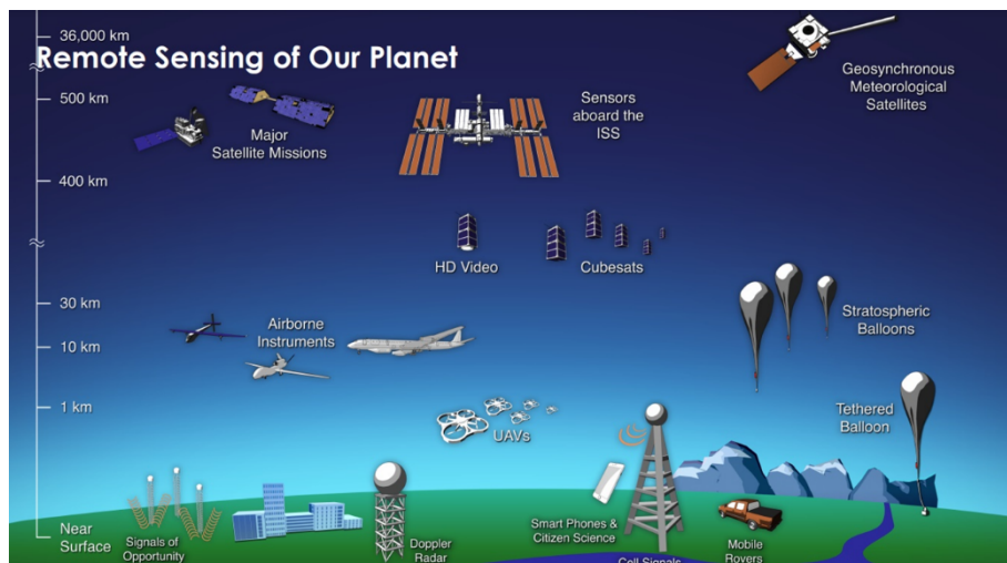
Fig. 1. Different types of remote sensors that obtain information from the Earth. Source: https://svs.gsfc.nasa.gov/30892
