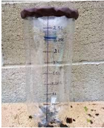
Fig. 6: Left: A homemade rain gauge. Right: Formula for calculating precipitation. It is important to mention that precipitation is measured in mm.
