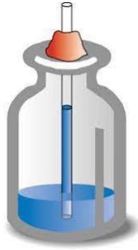
Fig. 4: A homemade thermometer
