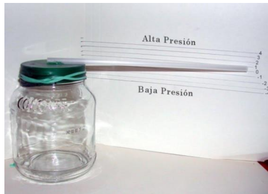
Fig. 5: A homemade barometer
