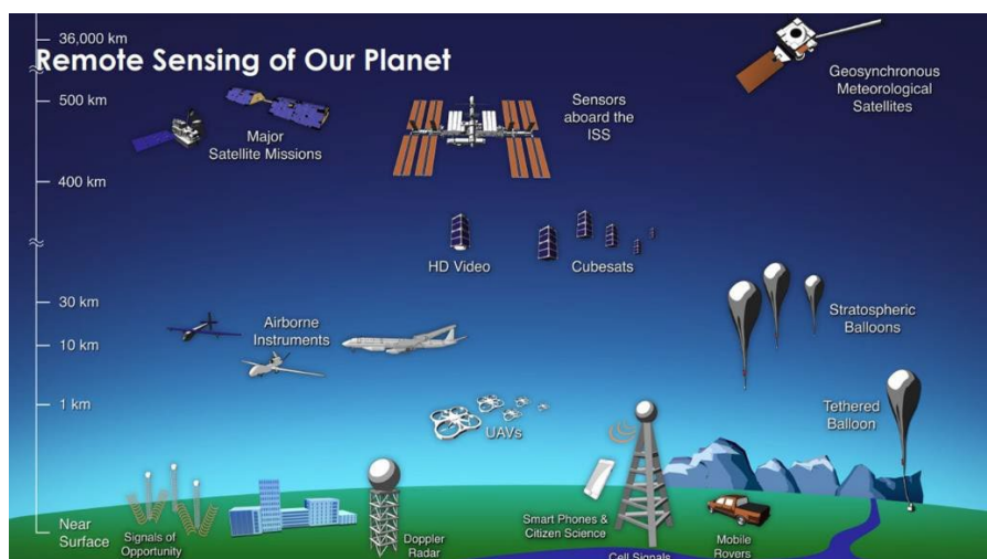
Fig. 1. Different types of remote sensors that obtain information from the Earth. Source: https://svs.gsfc.nasa.gov/30892
