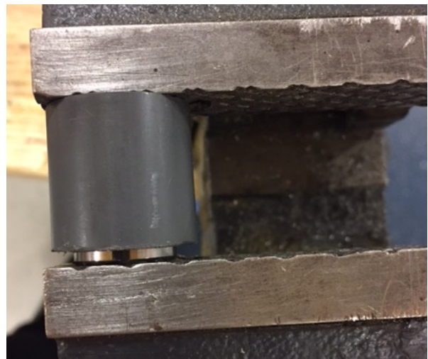
Position to press fit bearing with clamp
