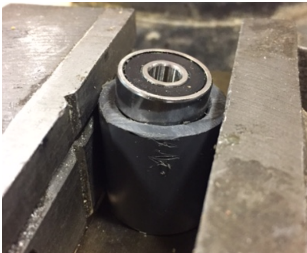
Position to tap bearing in with hammer
