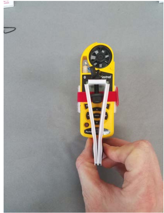
Attach the kestrel mount to the front of the aeropod.
