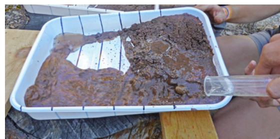
Figure 22- Students perform the flow investigation with the tray at a greater slope angle.
