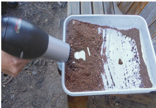
Figure 15- A student holds a hairdryer above the tray and behind the soil pile while directing the air down the slope of soil (wind investigation).
