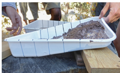
Figure 12- Students add a wood block under the soil end of the tray to increase the slope angle before doing the "advanced" rain investigation.
