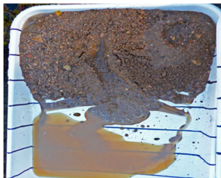
Figure 17- Examining a washout in the soil during the rain investigation. Mudslides, or landslides, in nature often occur after large rainfall events when soil becomes saturated with water and flows downhill.
