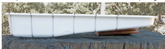
Figure 12- Students add a wood block under the soil end of the tray to increase the slope angle before doing the "advanced" rain investigation.
