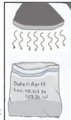
Figure 2, drying soil under heating lamp
