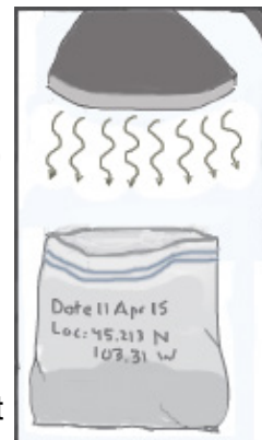
Figure 2, drying soil under heating lamp
